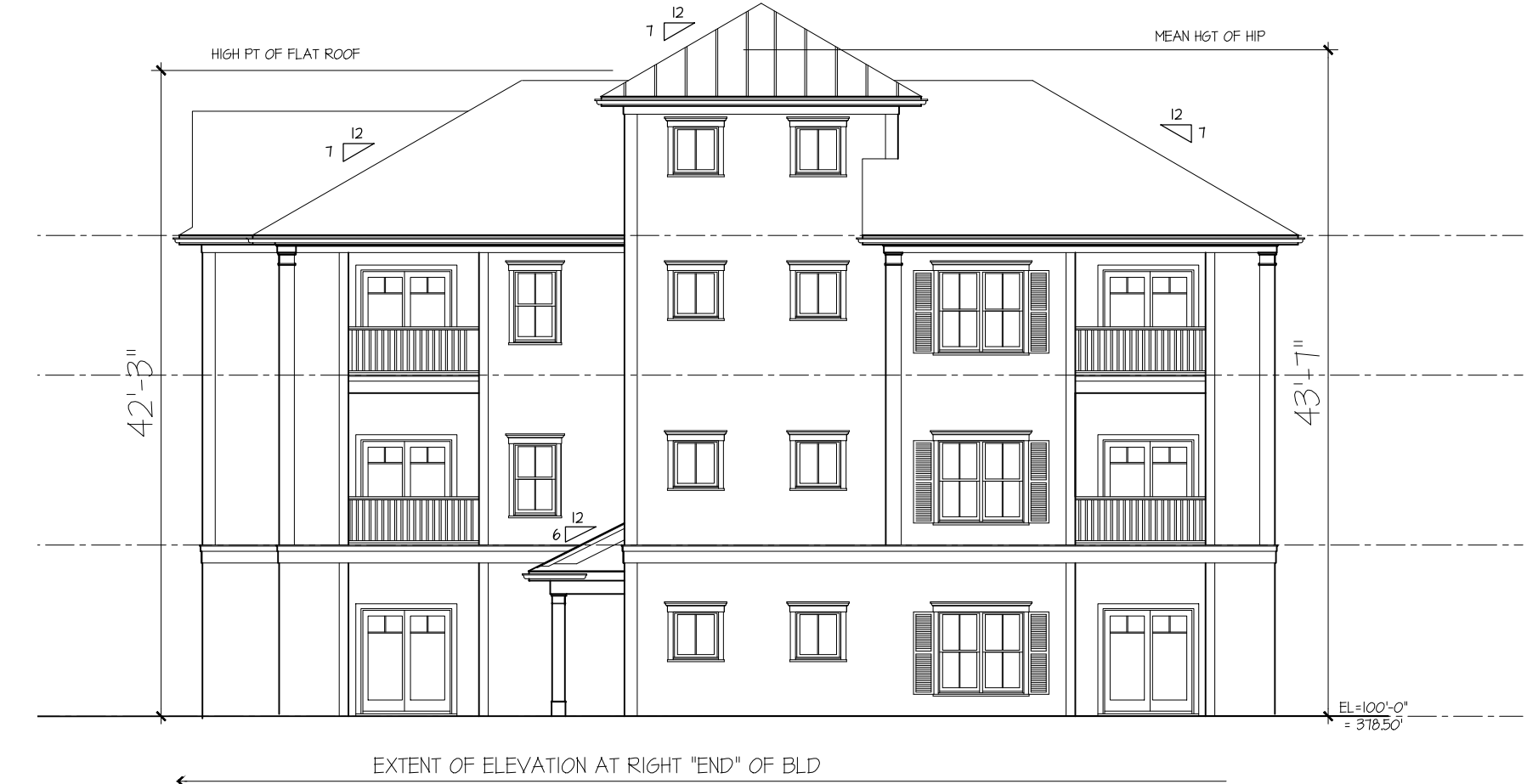
A RIGHT SIDE/END ELEVATION 3/32 = 1'-0"
