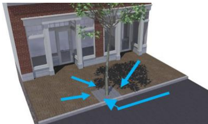
19. Tree Filter – External View. Credit: Stormtree
