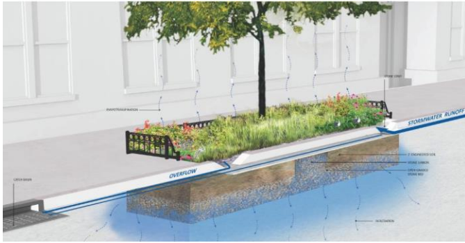
20. Flow-In Flow-Out Bioretention. Credit: Horsley Witten Group
