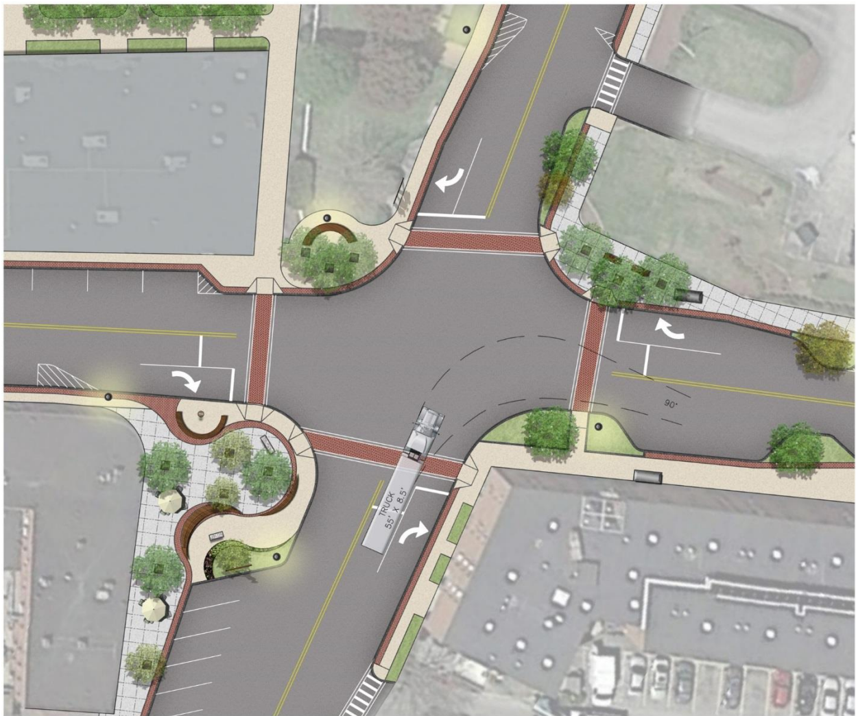
13. Close Up of Elm/Main Intersection, Bump Outs, and Turning Radii. Credit: Weston & Sampson
